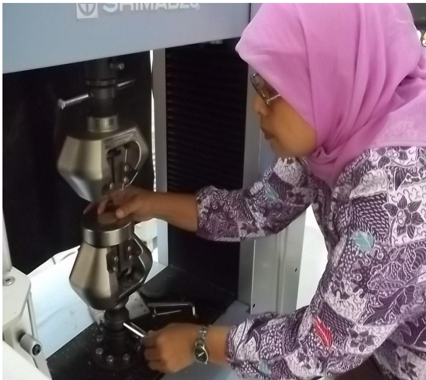
Gambar 20. Proses uji tekan/ Compression Test
